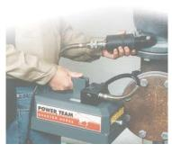
The Quarter Horse pump has a maximum operating pressure of 10,000 psi, which handles a wide variety of handheld hydraulic tools.
