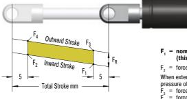
nominal force at 20 °C (this is the pressure figure normally used when specifying the gas spring)
