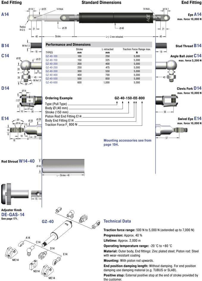
End fittings: They are interchangeable and must be positively secured
